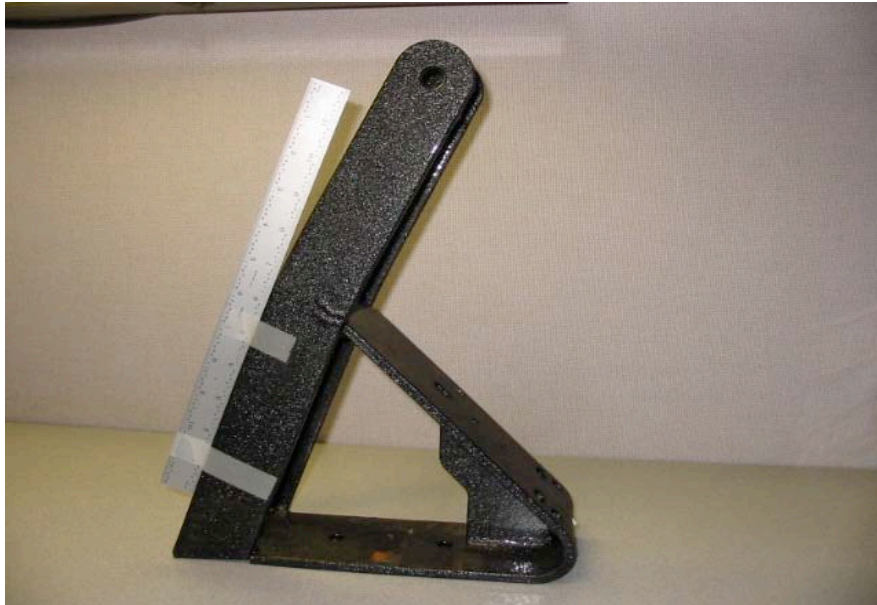
Fig. 7 - Bent winch stand upright supports after loading.
