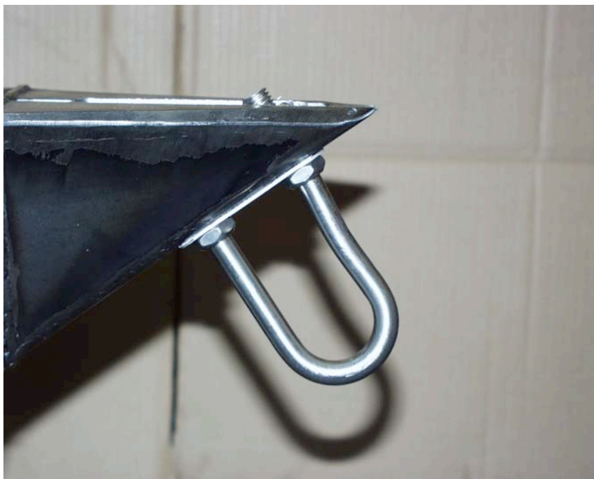
Fig. 4 - Bent bow eye after loading and contact with the SNAPPER mounting plate.
